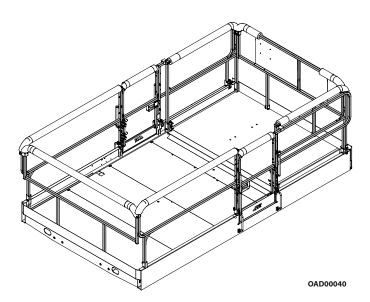
Platform Rail Padding provides bumpers to the top platform rails in order to prevent damage to the platform itself as well as objects it may come into contact with during operation.
