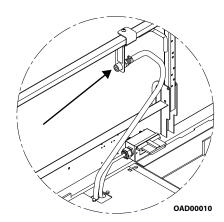
The 1/2 Airline is a fitting for air-powered tools that is mounted in the platform.
