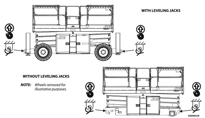
Figure 3-11. Lifting and Tie Down Chart (Sheet 2 of 2)
