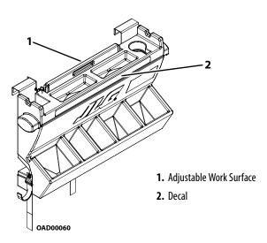
The Workstation offers an adjustable work surface and additional space for storage of tools and objects.
