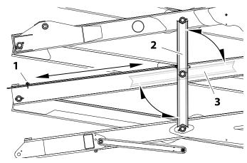
Figure 6-4. Scissor Arm - Safety Prop Assembly
