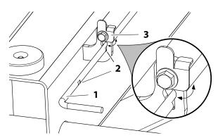
Figure 6-5. Safety Prop Actuator Rod
