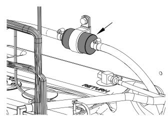
**NOTE:** Mounted inside fuel/hydraulic cabinet on left-rear cabinet wall behind fuel tank.
