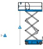
\* The metric equivalent of working height adds 2 m to platform height. U.S. adds 6 ft to platform height. \*\* CE/AUS markets: Two person maximum occupancy on all
