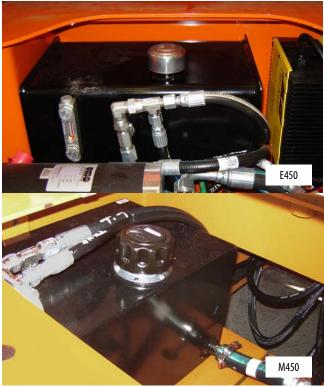
Lube Point(s) - Fill Cap Capacity - 4 Gal. (15.1 L)
