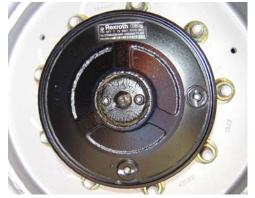
Lube Point(s) - Level/Fill Plug Capacity - 17 oz. (1/2 Full) Lube - EPGL Interval - Check level every 3 months or 150 hrs of operation; change every 2 years or 1200 hours of operation 6. Wheel Bearings
