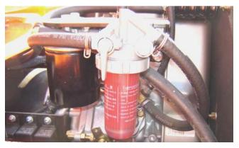
Lube Point(s) - Fill Cap Capacity - Refer to Engine Manual Lube - EO Interval - 3 Months or 150 hours of operation Comments - Check level daily/Change in accordance with engine manual.
