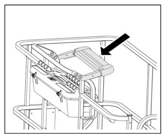
**NOTE:** If equipped, ensure the blue beacon illuminates when SkyGuard is activated.
