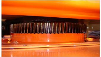
DO NOT OVERGREASE BEARINGS. OVERGREASING BEARINGS WILL RESULT IN BLOW-ING OUTER SEAL IN HOUSING.
